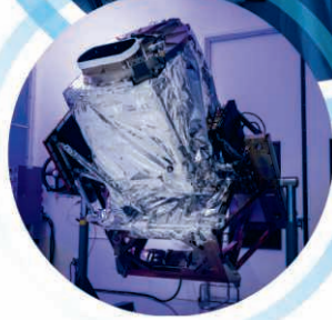
Tropospheric Emissions: Monitoring of Pollution (TEMPO) instrument
